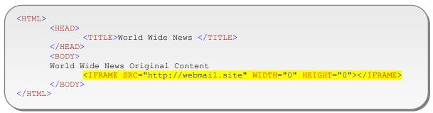
Figure 1: HTML page with an injected IFrame
